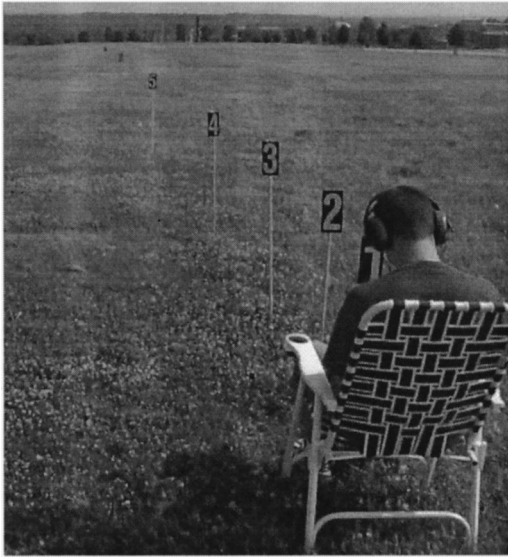
FIG. 2. Open field where the listeners judged the perceived distances of the speech sounds. Nine visual markers, numbered 1–9, were placed at locations 0.5, 1, 2, 4, 8, 16, 32, 64, and 128 m from the listener’s position and used as reference points for the listeners’ responses.
