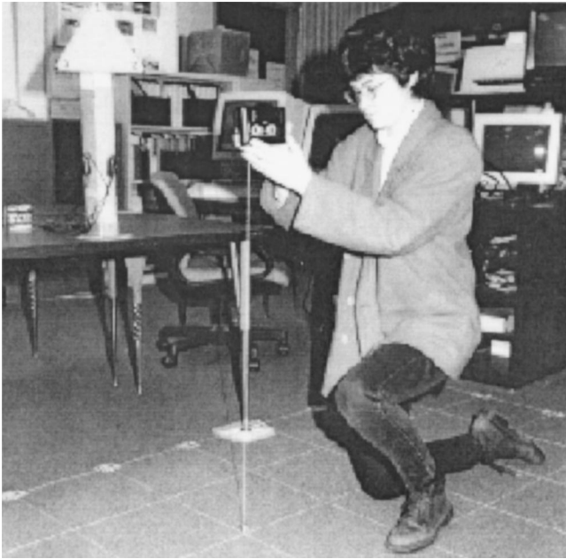
FIG. 12. Training the system. The compact sensor array is shown at the upper left corner of the figure. A tape recorder plays the sentence at a predefined height right above a floor grid point. A weight is used to guarantee vertical displacement between the grid point and the tape recorder.
