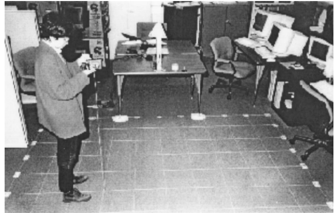
FIG. 11. The experimental setup. The compact sensor array is shown at the top of the pole standing on the edge of the center table. The intersection points on the grid on the floor mark the control points in the work space.
